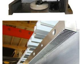
High precision gear racks, carefully installed and regulated by experienced worker with special purpose instrument, This assures smooth motion and long term reliability.
