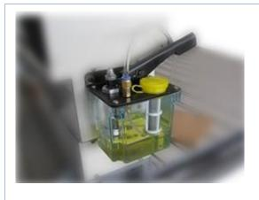
Central Lubricator: Easier to lubricate the Guide units regularly, just pull it gently and oil will go when it is needed.
