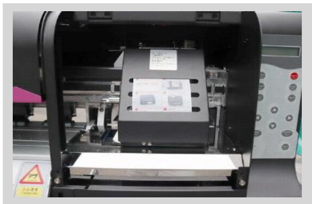
Epson I1600 / I3200-E1 print head in fine-made carriage
